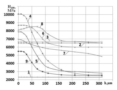
Fig. 3. Hardness distribution in the depth of surface layer at different thermal and chemical-thermal treatment: 1– steel 1:
