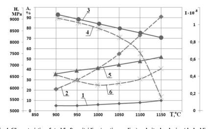
Fig. 4. Characteristics of steel 5 after nitriding (continuous line) and nitrohardening (dashed line): 1 - 2 - austenite content; 3 - 4 - microhardness of the surface layer; 5 - 6 - wear intensity after friction way 3 × 10<sup>3</sup> m
