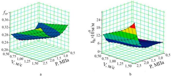
Puc. 5. Dependences of (a) the coefficient of friction ( $f_{TP}$ ) and (b) the intensity of linear wear ( $I_{h1}$ ) of material (90% PTFE + 10% silica gel) from loadings (P) and velocities (V) in time of friction interaction with steel
