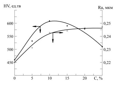
Рис. 4. Dependences of microhardness (HV) and roughness (Ra) of the steel surface from concentration of silica gel in PTFE before and after friction interaction with PC
