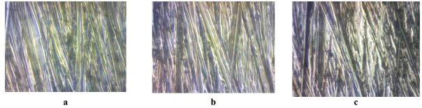
Fig. 3. Microphotographs of steel surface before (a) and after (b,c) frictional interaction with (6) PTFE and (c) PC based on PTFE and silica gel. Magnification in 400 times.
