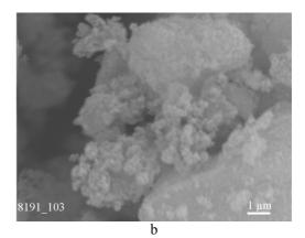
Fig. 1. Microphotographs of particles of silica gel
