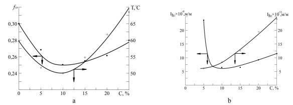
Fig. 2. Concentration (C) dependences (a) of the coefficient of friction (f<sub>TP</sub>), temperature on friction surface (T) and (b) the intensity of linear wear PC (I<sub>h1</sub>) and steel sample (I<sub>h2</sub>)
