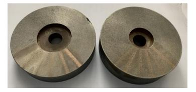
Fig. 1. Samples from cast iron SCh20 processed by the friction-mechanical method FANT
