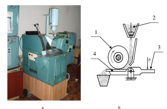
Fig. 3. Friction machine CMII-2 (a) and scheme of implementation of the process of abrasive wear (b): 1 - rubber roller; 2 - abrasive material; 3 - mechanism of load creation; 4 - a sample of the studied material.
