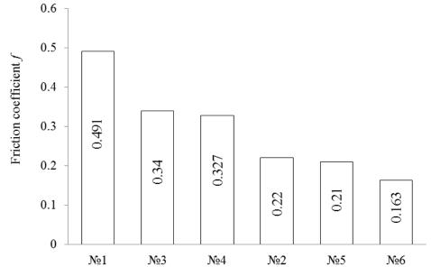
Fig. 6. Friction coefficient in the frictional interaction of a steel conjugate sample with polymer specimens:
