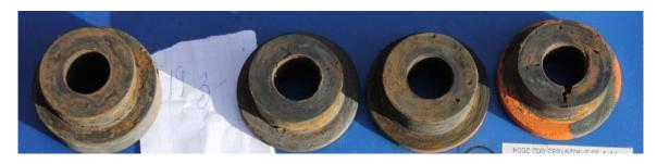
Fig. 9 - General view of experimental details of the upper lever after testing in paralelogram mechanism of cultivator
