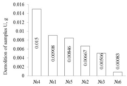
Fig. 5. The value of weight deterioration of polymer specimens with friction without lubricating on steel 45 (experimental conditions p = 0.5 MPa, v = 0.785 m / s)
