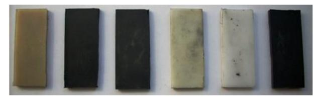
2 3 4 5 Fig. 2. General view of samples for determining relative abrasive stability: 1 – Nylon 66; 2 – PA-6-210X; 3 – PA6/6.6 R196-GF30; 4 – Kocetal GF705; 5 – Kocetal K300; 6 – CCPA-6-30
