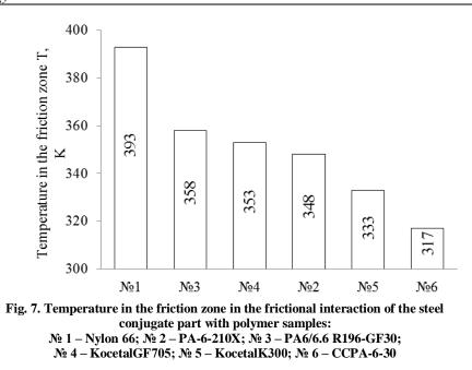
Stabilization of temperature T in the friction zone for all samples comes in the range of 8 minutes. (for Kocetal GF705) up to 40 minutes (Nylon 66) (Fig. 8).
