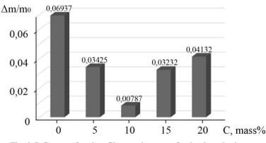
Fig. 2. Influence of carbon fiber on the wear of polyetheretherketone
