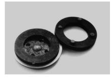
Fig.13. Billets for the thrust of the electric motor of the pump.
