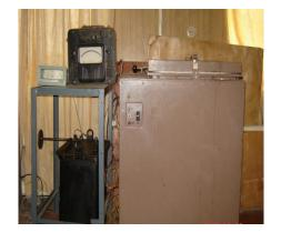
Fig.3 Electric furnace SSHO-3, Technical characteristics: Voltage, at 220; Power, kW- 6; Nominal temperature, °C - 380
