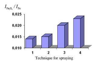
Fig. 4. The relative content of  $Fe_3O_4$  in coatings obtained using: (1) gas flame; (2) activated EAS in a reducing atmosphere; (3) activated EAS in an oxidizing atmosphere; (4) spraying with air.
