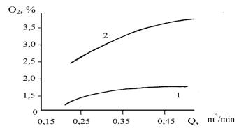
Fig. 3. Influence of the flow rate of spraying air on the oxygen content in coatings obtained by (1) mode 2 and (2) mode 3.
