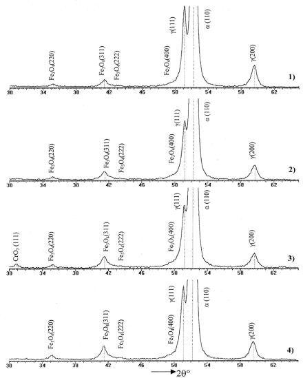
Fig. 5. Fragments of XRD patterns (CoKα) from surface layers of gas-thermal coatings obtained under modes 1-4.
