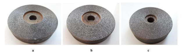
Fig. 1. Samples of cast iron SCH20, processed by the FANT friction-mechanical method with different  $\Delta l$ :  $a - \Delta l = 0,2 \text{ mm};$  $b - \Delta l = 0,4 \text{ mm};$  $c - \Delta l = 0,6 \text{ mm}$
