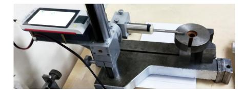
**Fig. 3.** Weighing a brass tool after FANT (a) and measuring the roughness of the machined surface (b)
