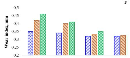
Fig. 3. Change in the wear index with an increase in the duration of the friction process in the turbine fuel Jet A-1: without additive (0) and at three different concentrations of FLNs (1, 2 and 5·10<sup>-4</sup>, % wt.)
