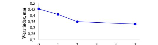
Fig. 2. Dependence of the wear index on the concentration of the LPF in the turbine fuel Jet A-1: the duration of the tribological tests is 5 min
