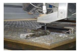
Fig. 8. Installation of a test piece on desktop of hydrocutting machine LSK-5-400
