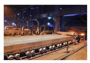
Fig. 4. Sintering cars of Zaporizhstal PJSC
