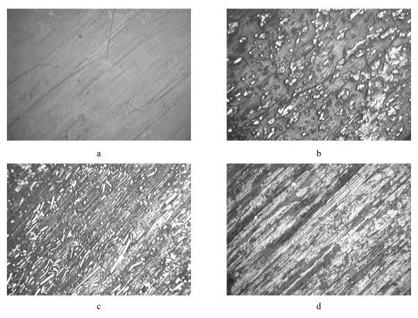
Fig. 1. Microstructures (×150) of friction surfaces of polytetrafluoroethylene (a) and basalt plastics based on it, containing: 10 (b); 20 (c), 40 (d) mass.% of basalt fiber
