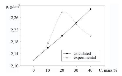
Fig. 2. Dependence of calculated and experimental density  $(\rho, g/cm^3)$  of polytetrafluoroethylene on basalt fiber content (C, mass.%)
