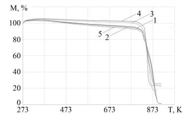
Fig. 3. Dependence of mass loss (M, %) on temperature (T, K) of polytetrafluoroethylene (1) and basalt plastics based on it containing: 10 (2); 20 (3), 30 (4), 40 (5) mass.% of basalt fiber
