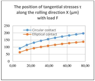
Fig. 7. Influence of microgeometry on the position of penetration of tangential stresses  $\tau$  in the subsurface zone of point contact along the depth z - ( $\mu$ m) for friction bearing units with increasing load F
