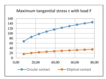
Fig. 6. Effect of microgeometry in the point contact zone on the change in tangential stress  $\tau$  for friction bearing units with increasing load F
