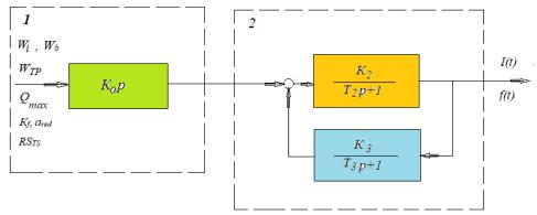
Fig. 1. Structural and dynamic scheme of simulation of tribosystems running-in processes
