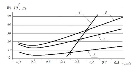
Fig. 2. Dependencies of the value of the input impact, when the loss of stability occurs (accelerated wear or burr), for different values of the sliding speed and tribological properties of the lubricating medium: 1 - MG-15B hydraulic oil; 2 - engine oil  $M-10G_{2K}$ ; 3 - transmission oil TS<sub>P</sub>-15K; 4 - the resulting curve for points that have the same loss of stability value
