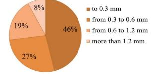
Fig. 1. Analysis of defects of parts of the "shaft" type according to the degree of wear
