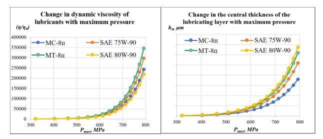
Fig. 3. Influence of the rheological feature (change in dynamic viscosity) of lubricants of different physical and chemical composition with increasing maximum pressure, taking into account the temperature in the contact zone T = 343 K for friction bearing units
