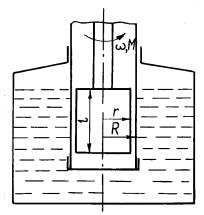
Fig. 1. General view of the rotational viscometer REOTEST 2.1.
