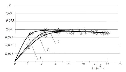
Fig. 13. Dependencies of the change in the friction coefficient during tribosystem running-in for different sliding speed values  $v_{sl}$ :  $1 - v_{sl} = 0,2$  m/s;  $2 - v_{sl} = 0,5$  m/s;  $3 - v_{sl} = 0,8$  m/s
