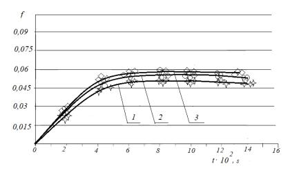
Fig. 11. Dependencies of the change in the friction coefficient during the tribosystem running-in for different load values N: 1 – N = 750 N; 2 - N = 1500 N; 3 - N = 2250 N
