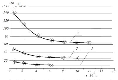
Fig. 8. Dependencies of the change in the volumetric rate of wear during the run-in of tribosystems for different values of the roughness of the friction surfaces Ra: 1 - Ra = 0,16 micron; 2 - Ra = 0,2 micron; 3 - Ra = 0,24 micron
