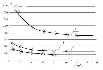
Fig. 4. Dependencies of changes in the volumetric rate of wear during the running-in of tribosystems with different lubricating media  $E_u$ : 1 - hydraulic oil MG–15V ( $E_u$ = 2,43·10<sup>14</sup> J/m<sup>3</sup>); 2 - motor oil M – 10G<sub>2 $\kappa$ </sub> ( $E_u$ = 3,6·10<sup>14</sup> J/m<sup>3</sup>); 3 - transmission oil TSp-15 $\kappa$  ( $E_u$ = 4,18·10<sup>14</sup> J/m<sup>3</sup>)
