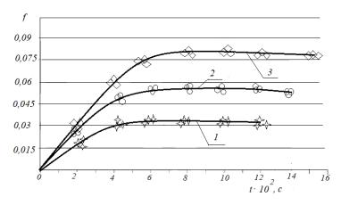
Fig. 9. Dependencies of the change in the friction coefficient during the running-in of tribosystems for different roughness values on the friction surfaces Ra: 1 - Ra = 0,16 micron; 2 - Ra = 0,2 micron; 3 - Ra = 0,24 micron
