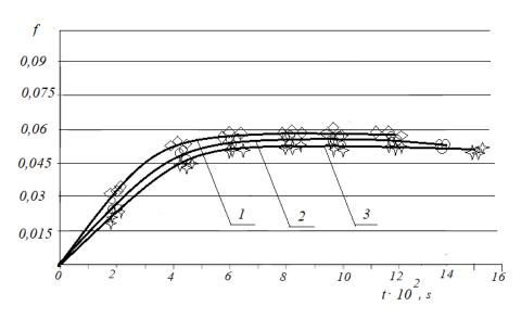
Fig. 3. Dependencies of the change in the friction coefficient during the running-in of tribosystems with different form factors  $K_{f}$ :  $1 - K_{f} = 5$  m<sup>-1</sup>;  $2 - K_{f} = 12,5$  m<sup>-1</sup>;  $3 - K_{f} = 20$  m<sup>-1</sup>
