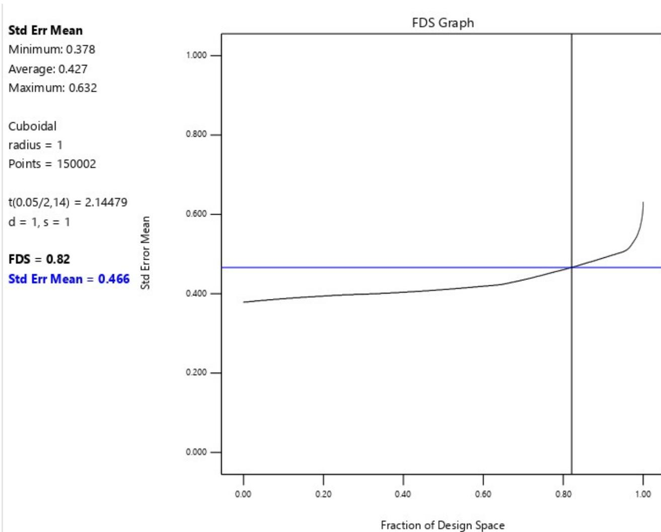
Figure 1: Fraction of Design Space (FDS) graph
