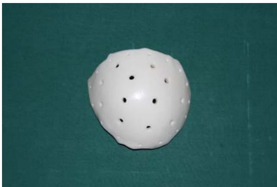
Figure 4 Using selective laser sintering (SLS) for rapid prototyping, both virtual models (defect and plate) were transformed into real models of polyamide. After a small manual processing, the plate fitted perfectly into the defect
