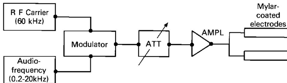
Fig 1: Schematic of high-frequency audiometer
