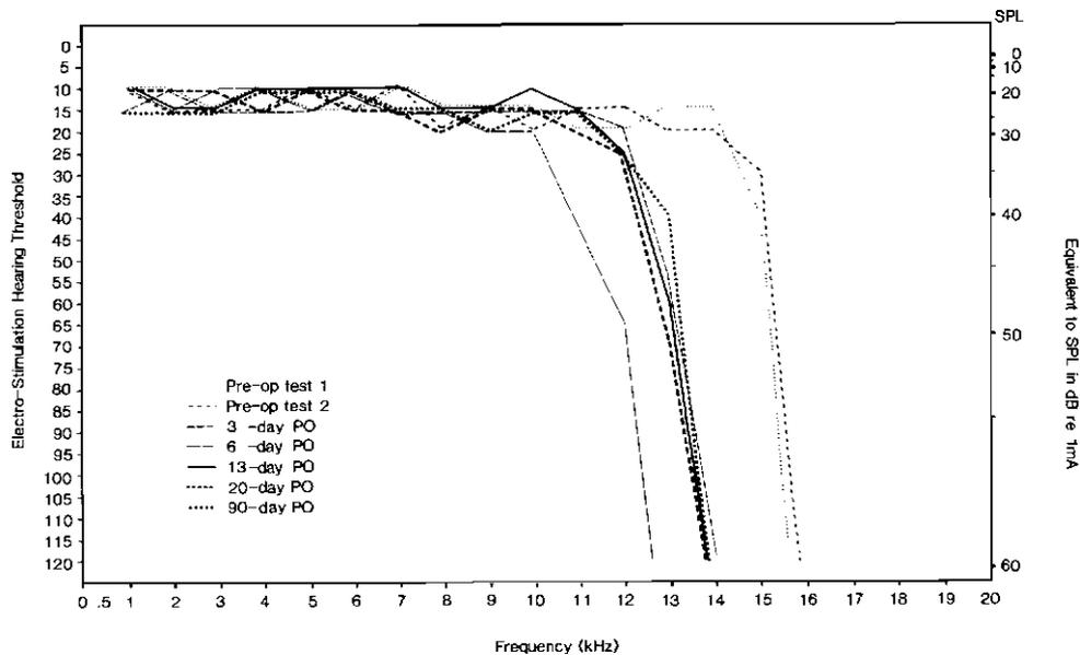
Fig 2: High-frequency threshold changes over time
