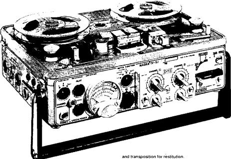
Four speed recorder: 15, 7;, 3; and 1; in/s. Two direct recording tracks and one FM track. Application as a precision sound level meter when a measurement microphone is connected.
