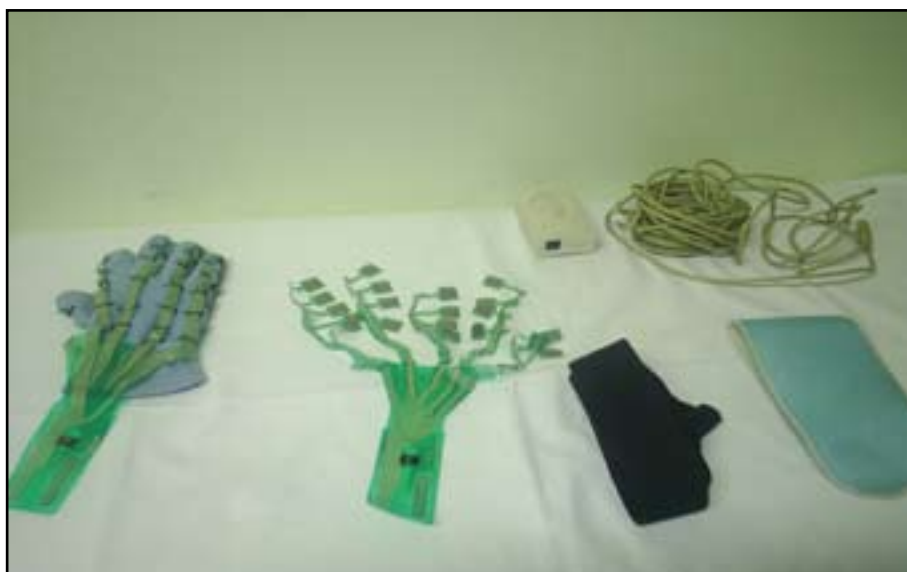
Figure 1: Photograph of grip system consisting of the sensors, cuff unit, straps and the connecting cable
