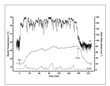
Fig. 1. Data from a 100 km cycle race. The course profile was measured using an uncalibrated air pressure sensor so that it recorded only relative changes in altitude. The heart rate transmitter was wired directly to the logger for accuracy. Data were logged approximately every 0.03 minutes to produce approximately 60 000 data points.
