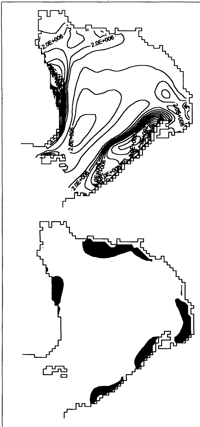
Fig. 12. Kinetic energy (in joules) for wind-driven circulation (a) and ratio between the spring ebb kinetic energy and wind-driven kinetic energy (b). Shaded areas represent ratios < 1 .
