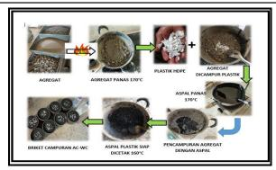
**Figure 2.** The process of mixing hot asphalt test specimens using plastic waste (source: research results in laboratory)
