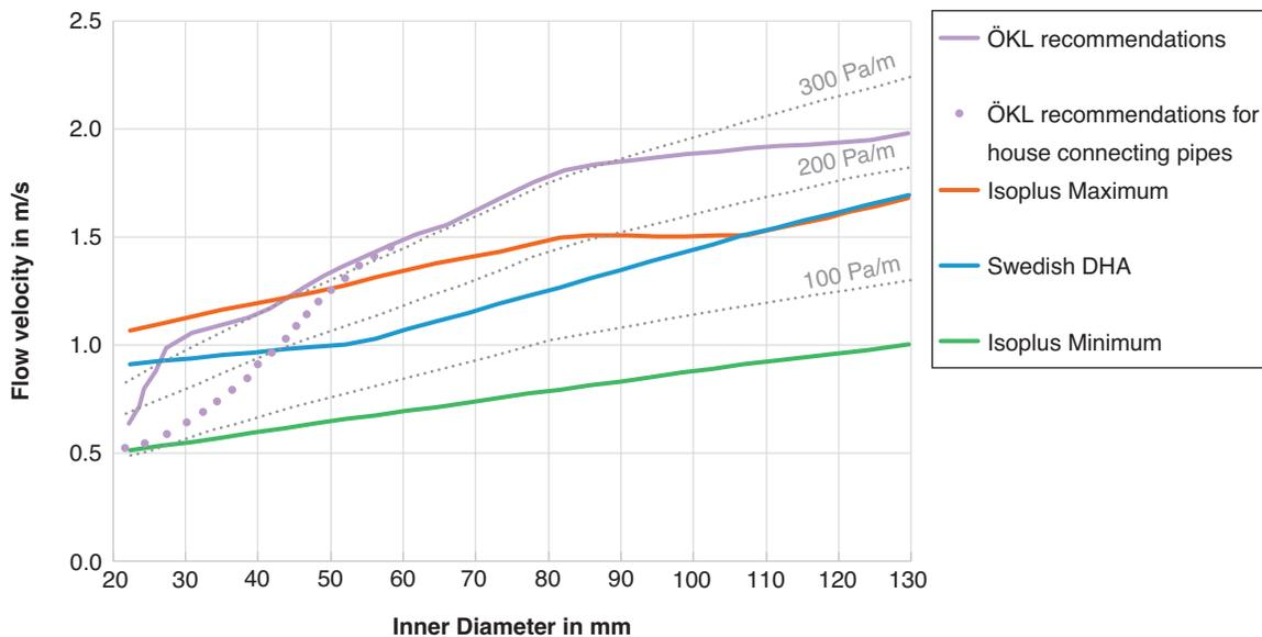
Figure 2: Different pipe design recommendations to ensure economic operation of the network
