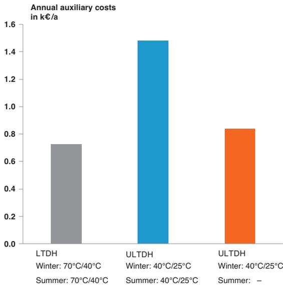
Figure 7: Resulting annual auxiliary costs distinguishing between conventional operation of LTDH network (grey), full year operation (blue) and a seasonal offline (orange) of ULTDH network
