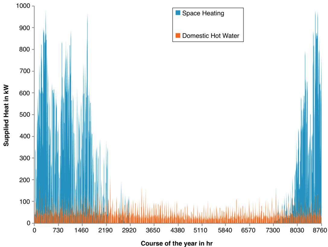
Figure 1: Calculated hourly heat load profile of the housing development “Zum Feldlager”, in blue the space heating demand, in red the domestic hot water demand
