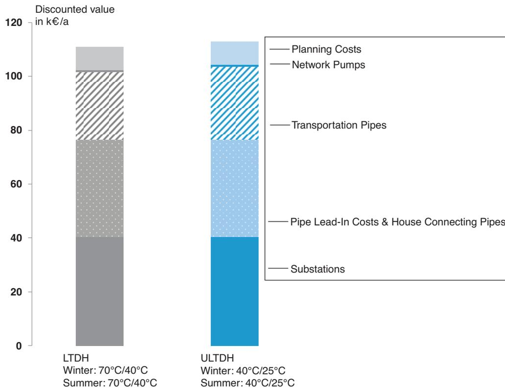
Figure 5: Net annual costs for the thermal network the thermal network LTDH (grey) and of ULTDH (blue)
