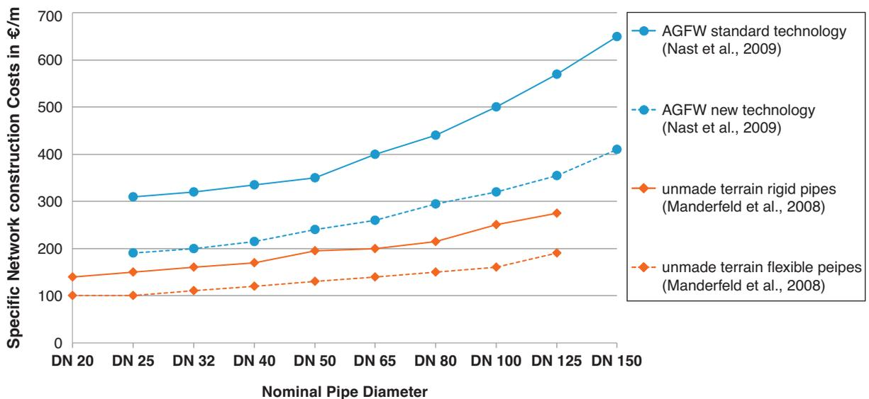
Figure 4: Specific network construction costs including construction costs and pipe material costs
