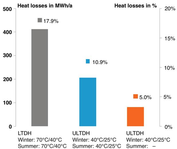
Figure 7: Heat distribution losses of the ULTDH and the LTDH network (with standard insulation)
