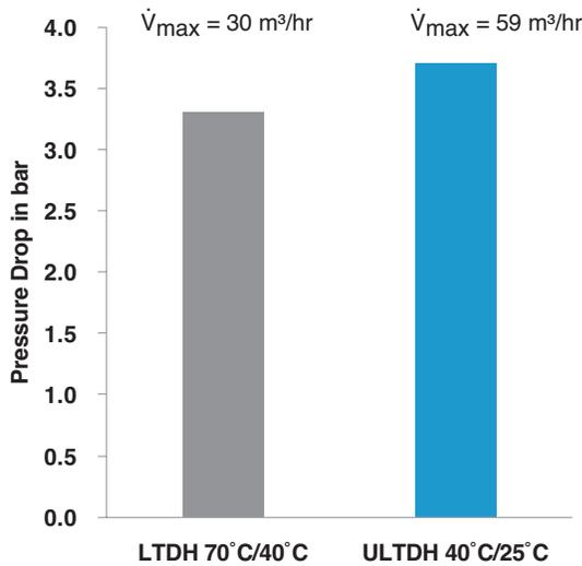
Figure 6: Pressure drop and needed volume flow at maximum heat load
