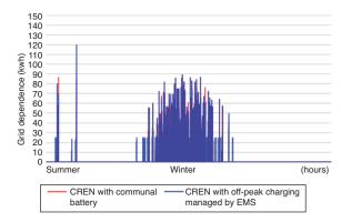
Figure 8: Hourly dependence of the community on the grid for two scenarios: community sharing individual resources as well as a communal battery all managed through a central EMS and the same community but without the communal battery and with off-peak charging managed by the EMS
