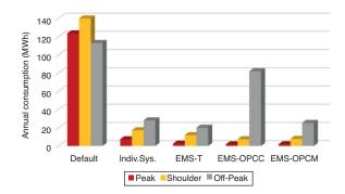
Figure 10: Comparison of peak, shoulder and off-peak electricity consumption for 5 scenarios: the default traditional connection to grid, individual generation +storage systems, community individual assets managed by central EMS, community assets + continuous off-peak charging managed by central EMS, and community assets + selectively managed off-peak charging managed by central EMS
