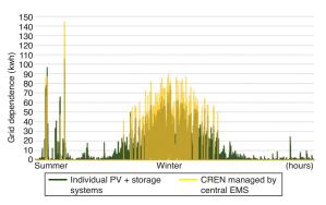
Figure 6: Hourly dependence of the community on the grid for two scenarios: individual dwellings each with its own, unshared PV + storage system, and the community sharing the generation and storage resources through a central EMS that balances all loads and available supply
