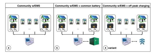
Figure 1: Scenarios modelled in detail: Community managed by central EMS, Community and communal battery managed by EMS, and Community and off-peak charging managed by central EMS. These scenarios correspond to scenarios 4, 5 in the previous paper. The last one is a variant of previous scenario 4
