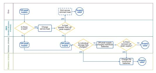
Figure 4: Flowchart summarising how the model allocates the overnight off-peak supply to either serve a load or charge the different storage assets in the electrical energy system of the CREN
