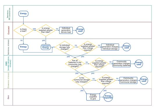
Figure 5: Flowchart summarising how the model allocates the energy supplied by individual PV systems to the different elements of the electrical energy system
