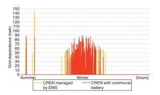
Figure 7: Hourly dependence of the community on the grid for two scenarios: community sharing horizontally the generation and storage resources through a central EMS and the same community setting but with an additional communal battery adding 500 kWh storage capacity
