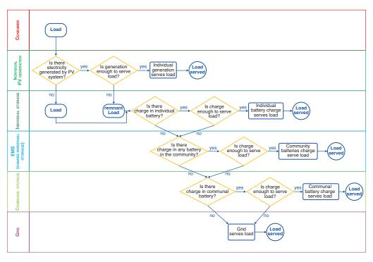
Figure 3: Flowchart summarising how the model uses the different elements of the electrical energy system to service the load of any individual dwelling
