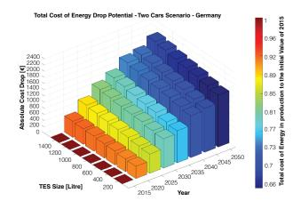
Figure 6: Drop potential in ATCE compared to the initial value of 2015 for all modelled years and TES sizes for a German singlefamily house in the 'Two Cars Scenario'
