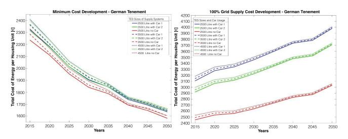
Figure 7: Development for ATCE per housing unit in a tenement (left) and development for ATGEC per housing unit (right)
