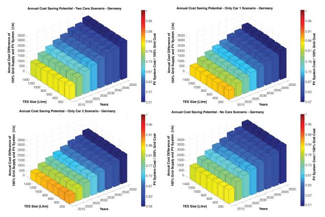
Figure A.2: Absolute and relative saving potential of ATCE compared to a 100% grid supply (ATGEC) for different TES sizes of the singlefamily system for the 'Two Cars Scenario' (top left), 'Only Car 1 Scenario' (top right), 'Only Car 2 Scenario' (bottom left) and 'No Cars Scenario' (bottom right)
