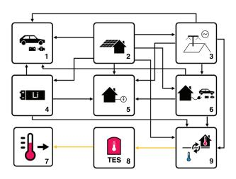
Figure 1: Structure of the PV prosumer model including conventional BEV (1), PV system (2), grid connection (3),stationary battery (4), residential electricity demand (5), BEV with V2H option (6), heat demand (7), thermal energy storage (8) and HP (9)
