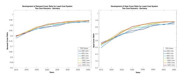
Figure 9: Development of DCR (left) and HCR (right) for all TES sizes and years for the 'Two Cars Scenario'
