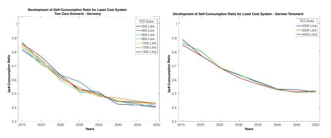
Figure 8: Development of SCR for single-family system (left) at the 'Two Cars Scenario' and for the tenement (right) for all years and TES sizes
