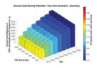
Figure 5: Saving potential of ATCE compared to a 100% grid supply (ATGEC) for all modelled years and TES sizes of a German single-family house for the 'Two Cars Scenario'
