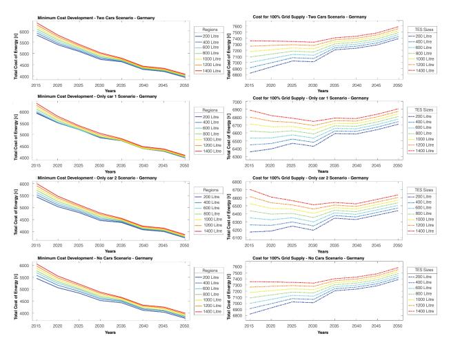
Figure 4: Development for ATCE for least cost system (left) and a full grid supply (right) for the different TES sizes and for 'Two Cars Scenario' (top), 'Only Car 1 Scenario' (center top), 'Only Car 2 Scenario' (center bottom) and 'No Cars Scenario' (bottom)
