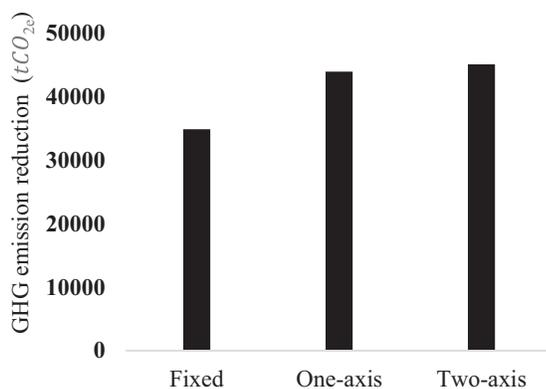
Figure 3: Net annual GHG emission reduction by fixed array and tracking systems
