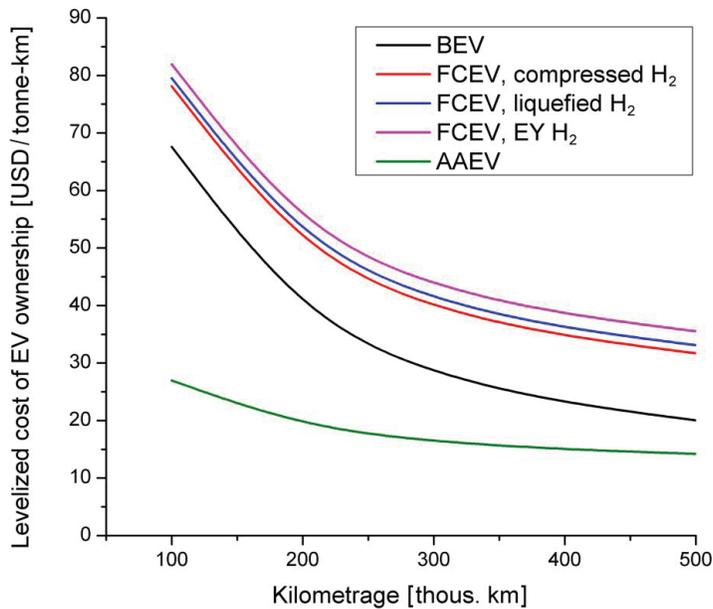
Figure 3: Levelized costs of EV energy carrier and. the power unit ownership, light duty commercial trucks, USD/tonne-km
