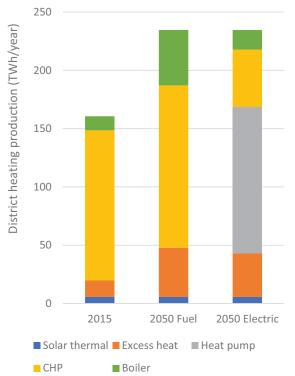
Figure 5: DH production divided on sources of heat for 2015, 2050 Fuel and 2050 Electric
