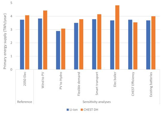
Figure 8: Results of sensitivity analyses to the 2050-Electric scenario for Li-ion and CHEST DH-Exchange
