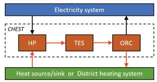
Figure 1: Conceptual illustration of system integration of CHEST with its main components; heat pump (HP), thermal energy storage (TES) and an organic rankine cycle (ORC).
