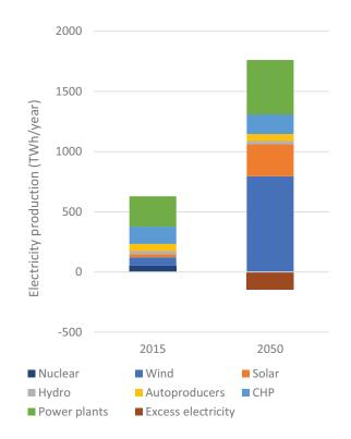
Figure 2: Electricity production divided into sources in 2015 and 2050 Fuel scenario.
