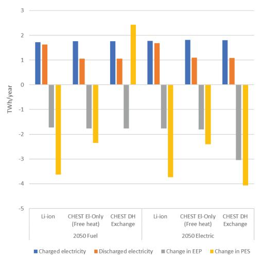
Figure 7: Main results of the three storage configurations in the Fuel-scenario and the Electric scenario. Results expressed as the change from the reference model without storage.
