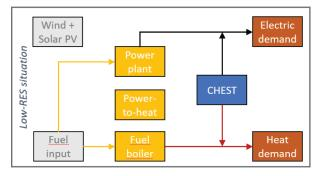
Figure 4: CHEST integrated in an electrified DH supply system in a situation with high production of wind and solar power (top) and one with low production (bottom).
