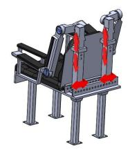
Figure 3: Adjustable prismatic joints
