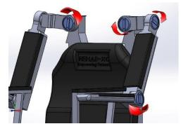
Figure 4: Rotation of each revolute joints.
