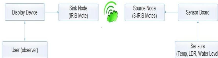
Fig. 2. Block diagram of the system
