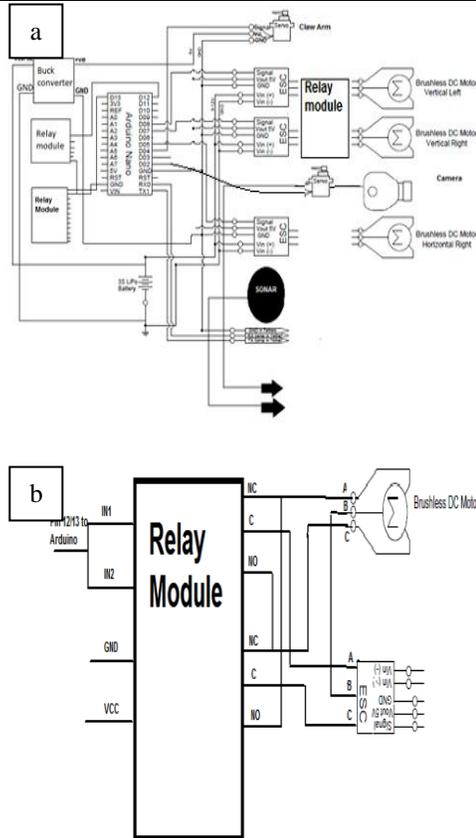
**Fig.4.**(a) Connection diagram of slave controller (b) connection diagram of thruster and relay module.
