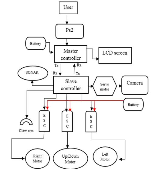
**Fig. 5.** Flow chart of UUV
