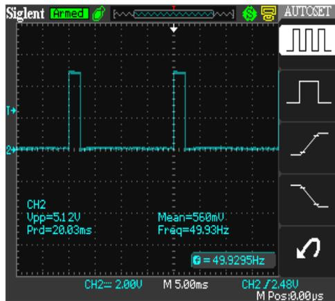
Fig.6. Shows the PWM of thrusters
