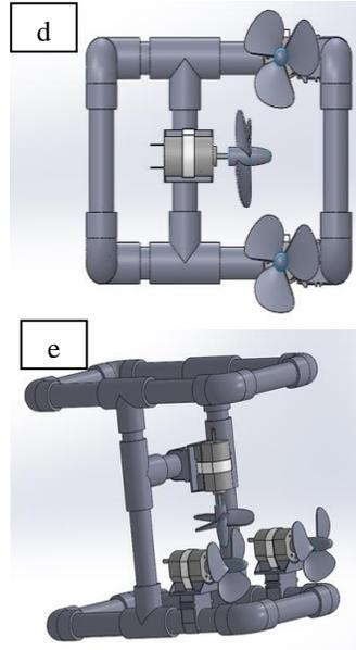
**Fig.1.** Thruster configuration (a) Top view of thruster (b) front view of thruster (c) Bottom view of thrusters (d) left view thruster (e) Right view of thrusters.
