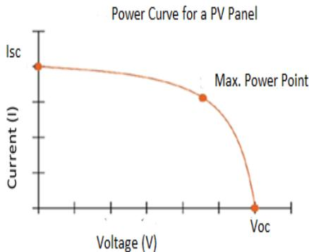
Fig 4: Power curve for PWM charge controller
