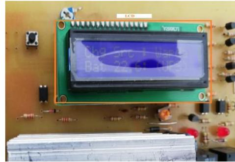
**Fig 15:** Charging of Battery through AC source
