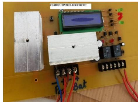
**Fig 16:** Solar Charge Controller
