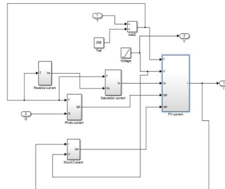
**Fig 6:** Grouped Subsystem of PV module
