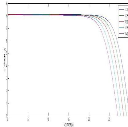
Fig 9: I-V characteristics under varying temperature
