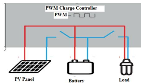
Fig 1: PWM charge controller
