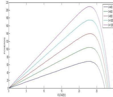
Fig 8: P-V characteristics under varying irradiance
