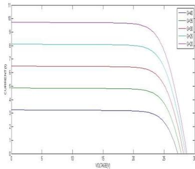
Fig 7: I-V characteristics under varying irradiance
