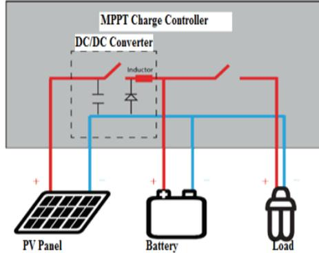
Fig 3: MPPT charge controller
