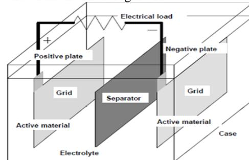
**Fig 11:** Lead Acid Battery
