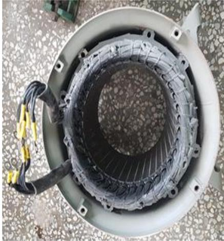
Fig 8: The Standard stator from a Cummins BCI-184F machine
