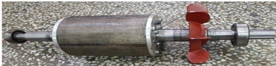
(c) Assembled rotor with shaft, fan and bearing before machining
