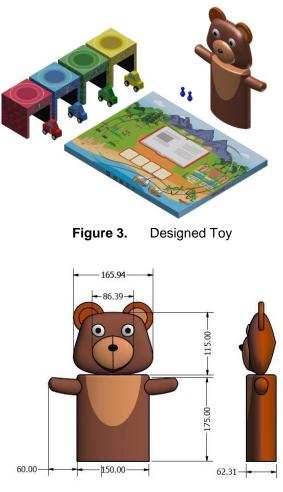
Figure 4. Hand Puppet Dimension in mm
