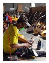
Figure 2. Attaching the wire to the frets using a hammer and glue
