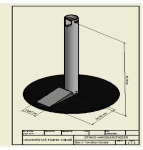
Figure 3. Engineering drawings of 3D ergonomic design of hand sanitizer dispenser stand
