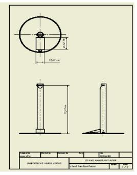
Figure 4. Engineering drawings of 2D ergonomic design of hand sanitizer dispenser stand
