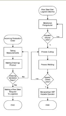
Figure 5. SOP Welder
