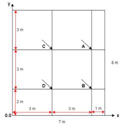
Figure 2. Point of Lighting Measurement
