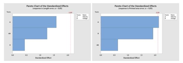
Fig. 3. Pareto Chart of Length error and Printed area error
