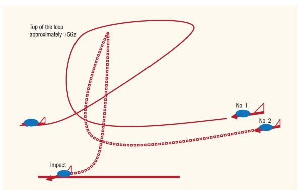
**Figure 2:** The construction of the flight profile which may have led to the fatal crash because of possible pilot incapacitation due to a gravity-induced loss of consciousness (G-LOC). Note the figure is not mathematically accurate.
