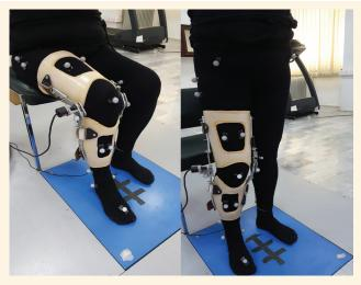
Figure 3: Photographs showing the knee range of motion testing in the transverse plane in a sit-to-stand test with a knee orthosis.
