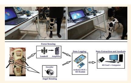
Figure 2: Photographs showing how the interactive shearing force between the limb and the orthosis in a sit-to-stand task was measured using different instruments.
