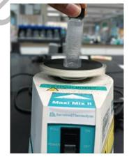
Fig. 5- Preparation of demulsifier DB using Barnstead Thermolyne Maxi Mix II Vortex Mixer
