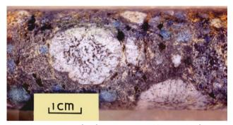
Figure 69. Syneresis shrinkage patterns in Tennant Creek coarse porphyroids have associated orebodies.
