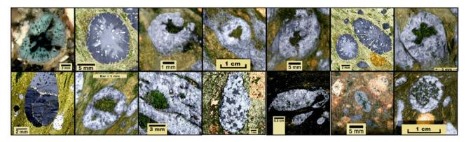
Figure 63. Polymeric silica accretions from Great Western porphyroid, Tennant Creek, have crystallised to quartz.
