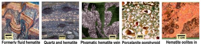
Quartz and hematite Ptygmatic hematite vein Porcelanite porphyroid Hematite oolites in accretions in BIF in former chloritic mud from Wittenoom Olympic Dam granite
