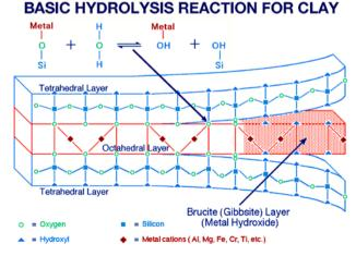
**Figure 48.** The external surfaces of natural clay platelets are fully hydrated. In the marine environment, further hydrolysis can therefore only progress inwardly from the edges of the platelets (within the octahedral layers).
