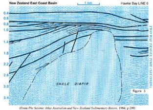
**Figure 37.** Seismic surveys<sup>15</sup> record a large intrusive shale mass in Hawks Bay, New Zealand.
