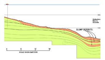
**Figure 34.** Massive submarine slope failure involves liquefaction of large volumes of sediment. Lehner<sup>12</sup>, 1969, fig. 45.
