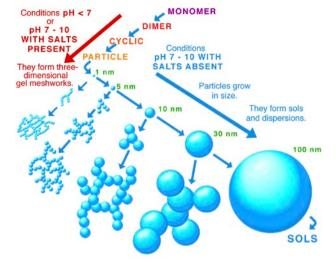
**Figure 47.** This diagrammatic representation of the growth of natural silica particles is re-drawn from Iler<sup>8</sup>, 1979, p. 174.
