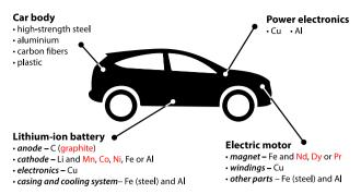
**Figure 7.** Most relevant materials used in different parts of battery electric vehicles. Those defined as critical are highlighted in red.
