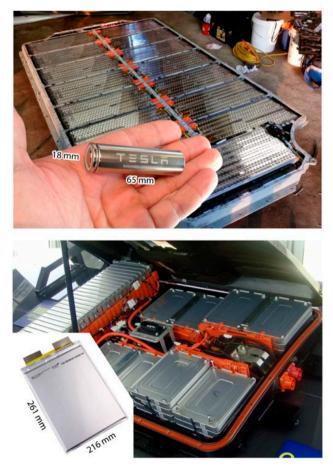
**Figure 6.** Individual cells for BEVs and their final assembly in the pack: Tesla (cylindrical, top) and Nissan Leaf (puch, bottom).
