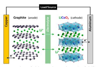
**Figure 5.** Scheme of a lithium ion battery, where  $Co^{4+}/Co^{3+}$  half reaction occurs at the cathode and redox-promoted intercalation of lithium in graphite takes place at the anode.
