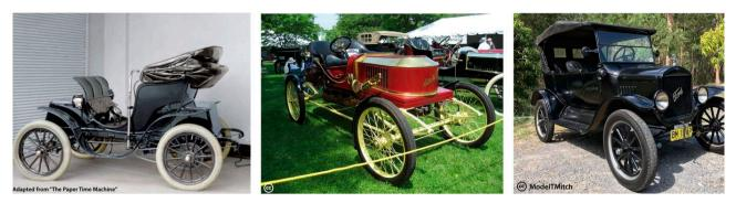
Figure 1. From left to right, examples of electric, steam and internal combustion engine cars of the early 20th century (1906, 1908, 1925, respectively).
