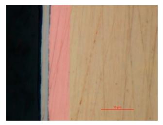
**Figure 4.** Cross section of typical galvanic deposition analyzed with optical microscope. From left to right it is possible to distinguish: brass substrate, copper, nickel and gold finishing. Before the cut of the sample an additional layer of nickel was deposited on gold to preserve its integrity and sharp edge during the lapping process.
