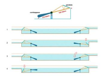
Figure 27. Operation of the counterweight system designed to support one *braccio* of water.
