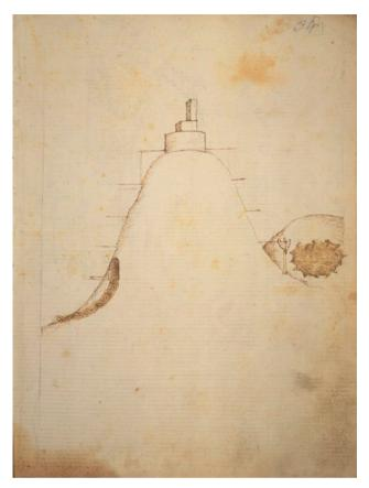
**Figure 24.** Mariano di Iacopo, called il Taccola, *De ingeneis*, Biblioteca Nazionale Centrale di Firenze, Ms. Palat. 762, c. 34r: method for digging a tunnel for the passage of canals and aqueducts.
