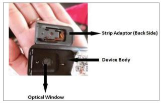
Fig-5: Optical window exposed after sliding strip adaptor from the device body
