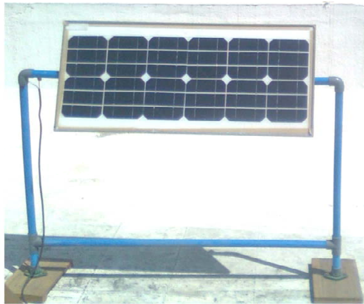
Figure 12. SOLKAR PV panel (Model # 3712/0507) with tilting stand arrangement to change insolation levels
